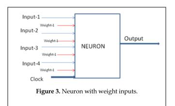
Figure 3 Shows 4 inputs referred to the weights of the connection between other neurons and our neuron. Every weight is in relation with each dendrite. It is necessary a clock signal to make synchronous the system.
