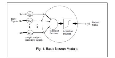
The common mathematical model of a neuron is shown in Figure 1. According to the above, the net input to the ith unit of the next layer from the jth node can be written as:
